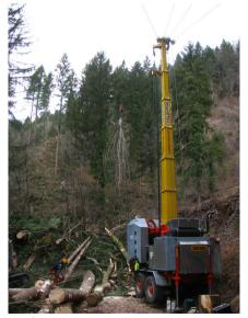
Figure 3 The tower yarder at work, during inhaul
