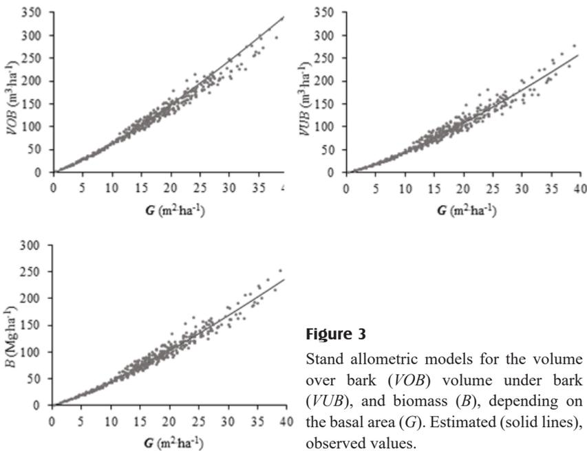
**Figure 3** Stand allometric models for the volume over bark (*VOB*) volume under bark (*VUB*), and biomass (*B*), depending on the basal area (*G*). Estimated (solid lines), observed values.
