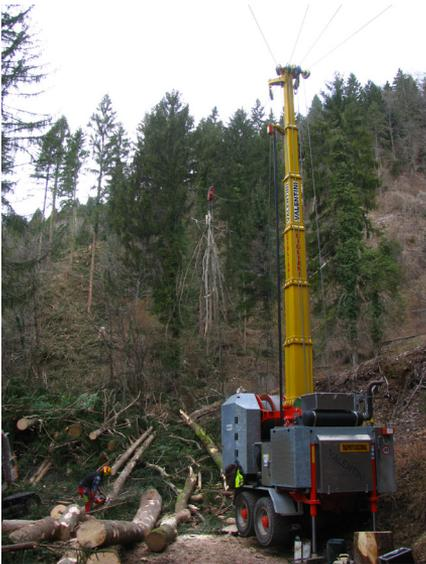
**Figure 3** The tower yarder at work, during inhaul
