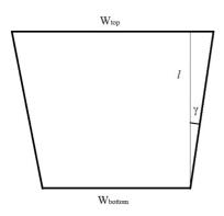
**Figure 2** Lateral angle  $(\gamma)$  of a reach with trapezoidal shape
