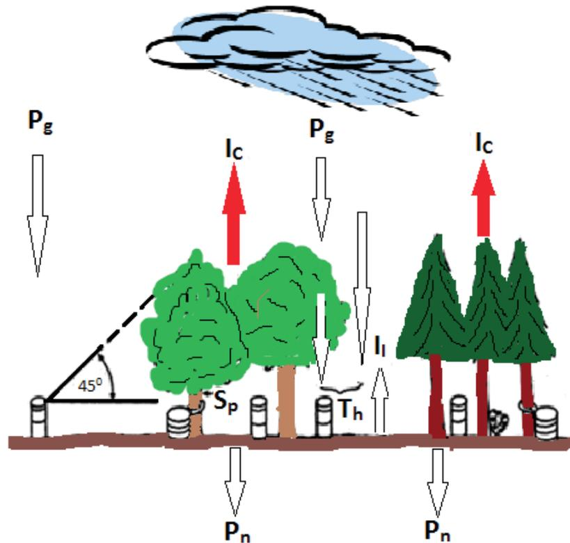
**Figure 3** Elements of interception, where IC - interception of vegetation, II - interception of dead cover,  $P_g$  - rain falling on the open area,  $P_n$  - net rainfall,  $S_t$  - stemflow and  $T_h$  - throughfall (Brooks et al. 1997)
