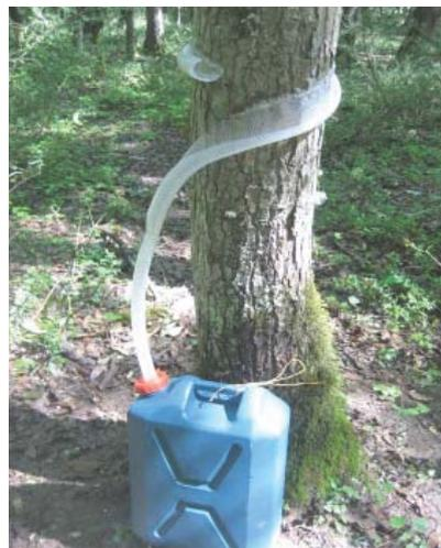
**Figure 4** A stemflow (SF) collector
